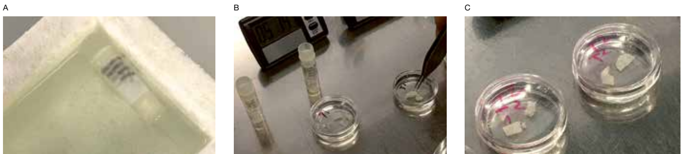
Fig. 4: Thawing Procedure. A) In Water Bath; B, C) in Thawing Solution 1 and 2.
