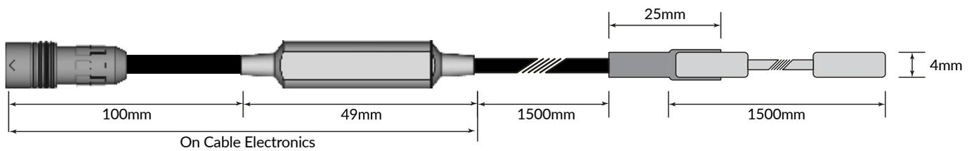
Supplied with 1.5 M flexible mineral insulated cable
