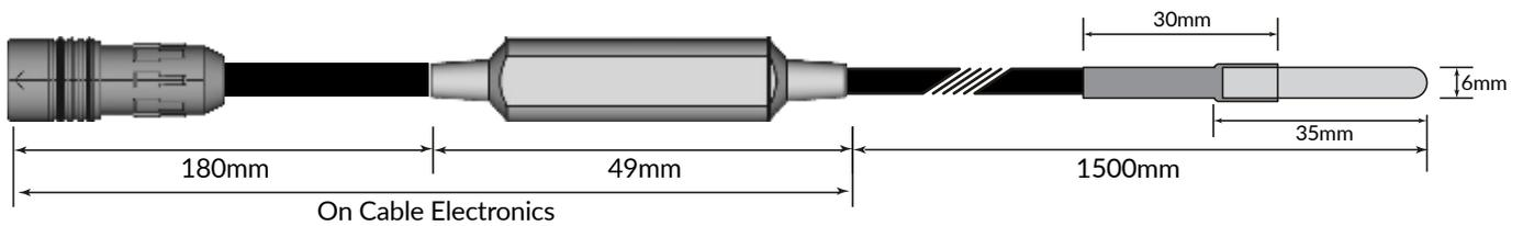
Supplied with 1.5 m 3 core FEP cable
