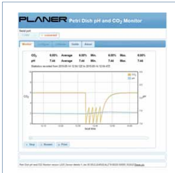
Figure 3. Monitoring of both the culture chamber CO 2 levels and corresponding predicted pH following multiple lid openings in a benchtop incubator.
