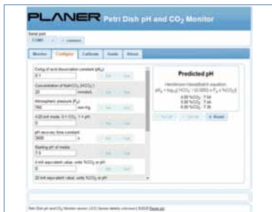
Figure 2. Configure tab of the Petri dish pH / CO 2 application allows input of parameters used to determine pH in an established culture system
