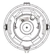
Shock absorbing foam in the PPSC helps prevent damage to the dewar. Illustration shows top view of the tank in the PPSC.
