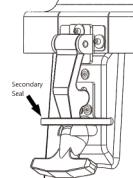
The rubber latch design allows the use of a zip tie, vet seal, safety seal, etc. to ensure integrity of product shipped.
