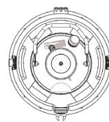
Shock absorbing foam in the PPSC helps prevent damage to the dewar. Illustration shows top view of the tank in the PPSC.
