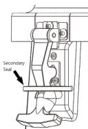
The rubber latch design allows the use of a zip tie, vet seal, safety seal, etc. to ensure integrity of product shipped.
