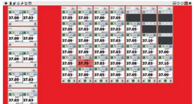
Display alerts and manage alarm notifications for any incubator connected to the system
