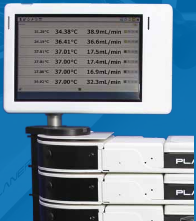
PIMSsolo unit mounted on a CT37stax™ system
